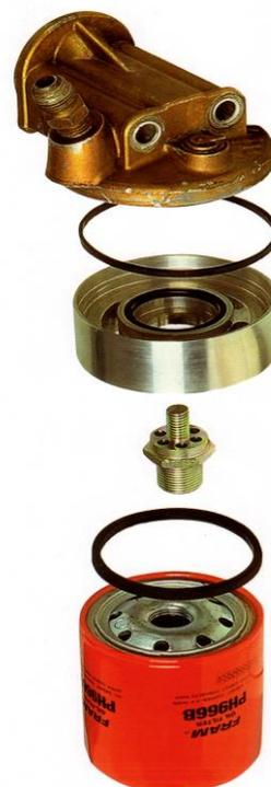
Remove the bowl which contains the original oil filter element and place to one side. Remove the old rubber seal which sits in the groove in the filter head. This may be difficult to see and it often seems as though there is no seal as they become hard and compressed with age, but it is important to replace this seal in order to ensure a leak-proof installation.
